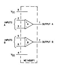
CHARACTERISTICS SUPPLY VOLTAGE: V<sub>CC</sub> +18 V DC MAX VEE -18 V DC MAX PUT DIFF VOLTAGE: ±30 V MAX INPUT COMMON MODE VOLTAGE: ±15 V MAX (1) OUTPUT SHORT CIRCUIT DURATION: CONTINUOUS (2) INPUT RESISTANCE: 300 kΩ MIN, 2.0 MΩ MAX OUTPUT RESISTANCE: 750 TYPICAL VOLTAGE GAIN: 15 MIN
